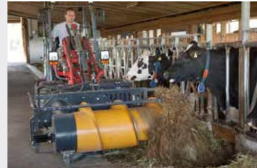
The standard feed refresher is equipped with a three-point attachment. The standard application can not only be used on a tractor, but also on farm loaders, wheel loaders and on front loaders.
