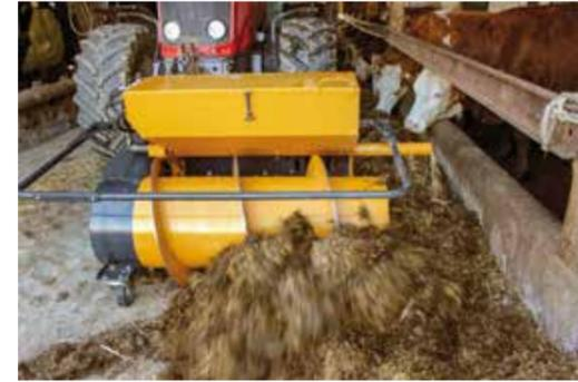
Clean pushing of feed with ideal loosening of the silage.
